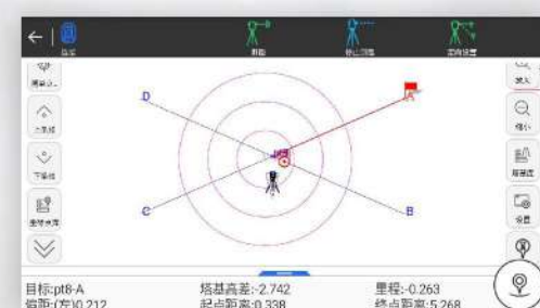
Tower footing stakeout
